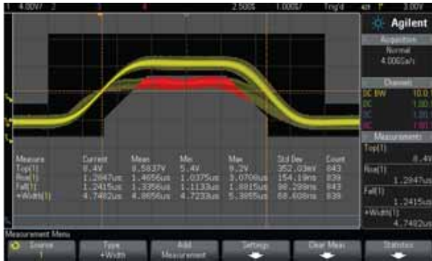
Figure 3: ARINC 429 “1’s” pulse mask test with parametric measurements.
