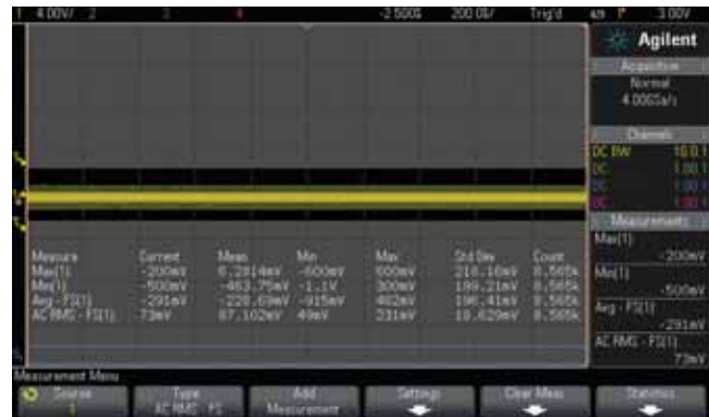
Figure 5: ARINC 429 “null” mask test with parametric measurements.
